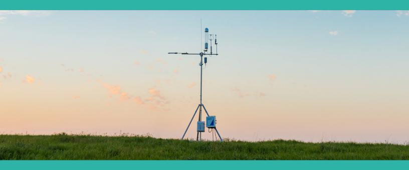
Gas analyzers feature low noise, high precision, long-term stability, and low power consumption. The SmartFlux System provides exquisite analysis of gas, wind, and biomet data, for fully processed flux results in real time. Systems include the leading eddy covariance software, including EddyPro® Software to compute results.
