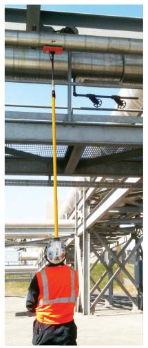
Lightweight telescopic pole allows easy access to hardto-reach areas and eliminates the need for scaffolding.
